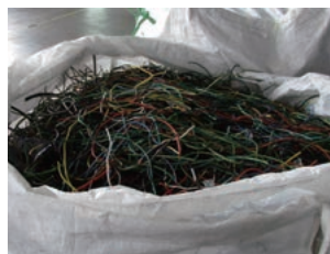
Shredded electric wire
