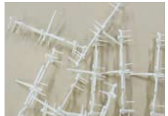
Un-needed runner pieces after injection molding
