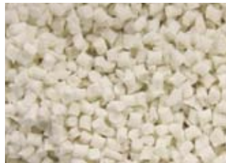
Resin pellet containing a mix of virgin and recycled materials
