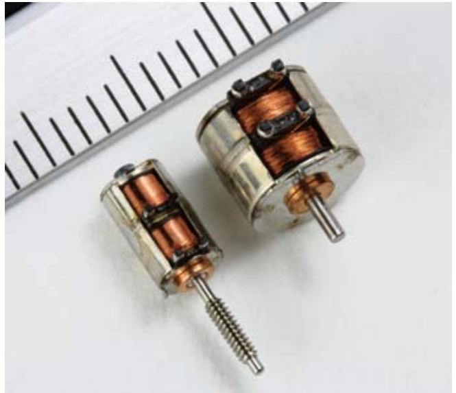
Ultra-small permanent magnet (PM)-type stepping motor with high resolution (Left 3mm dia, right 6mm)
