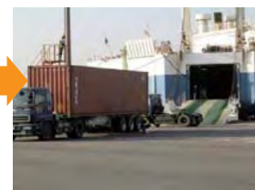
RORO ship (Roll On & Roll off ship) High-speed ferry that allows loading and unloading truck containers as they are without using large-sized harbor cranes to save time.
