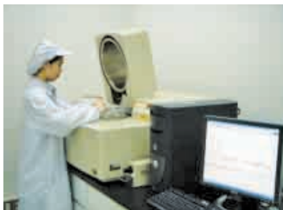
Testing procedure using XRF spectroscope at the Bang Pa-in Plant in Thailand
