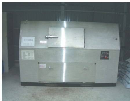
Perishable waste processor (Hamamatsu Manufacturing Unit)
